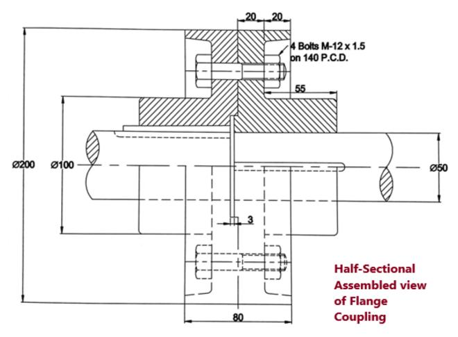
Annexure -6 (Assembly to Detailed Sectional Drawing)
