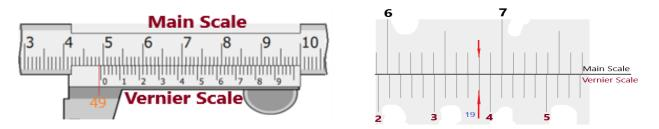
Observe the above figures of a vernier caliper carefully and fill the blank spaces with key words and specific numerical values.
